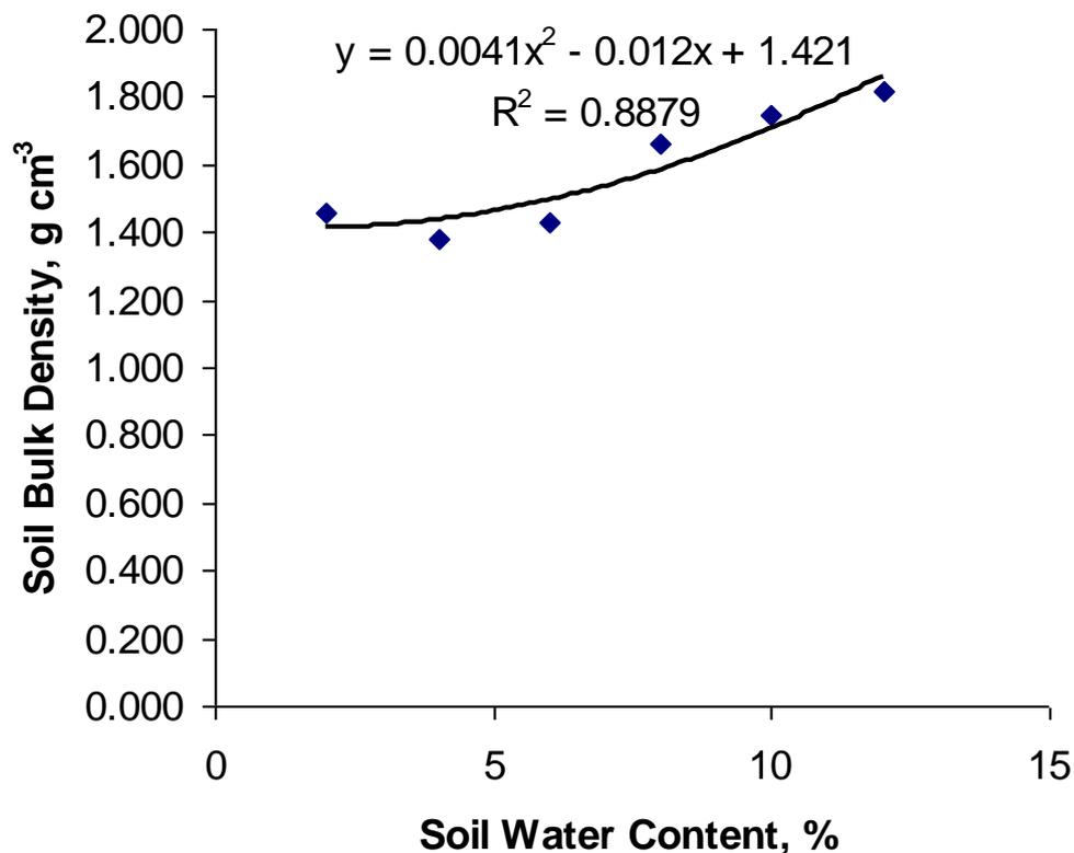
**Figure 1.** Soil compaction tests determination through the standard proctor test.
